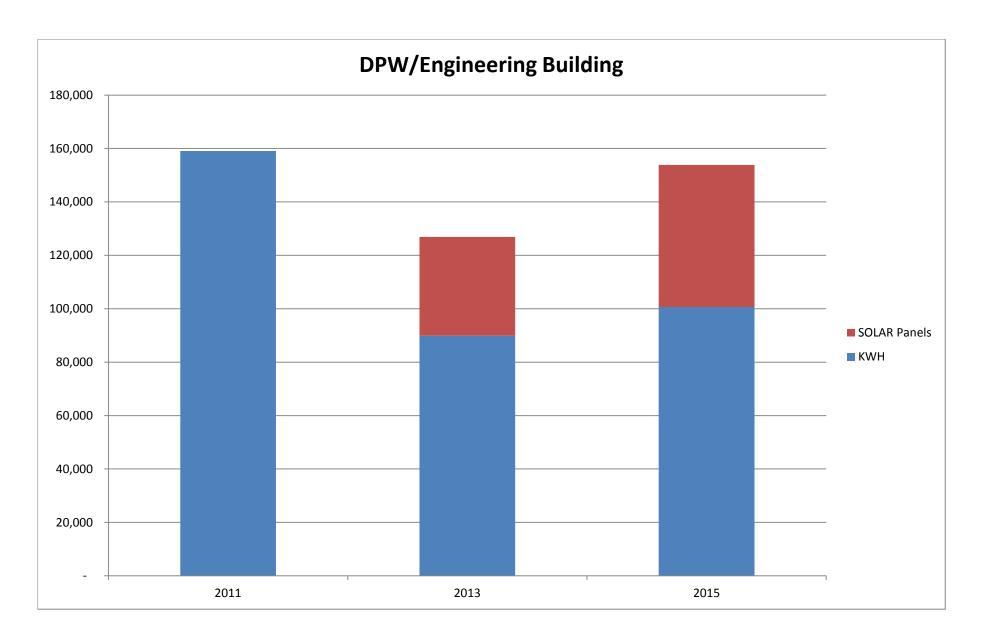
Significant reduction in KWH since 2011 due to the installation of Solar Tubes and Solar Panels at the DPW/Engineering building.
