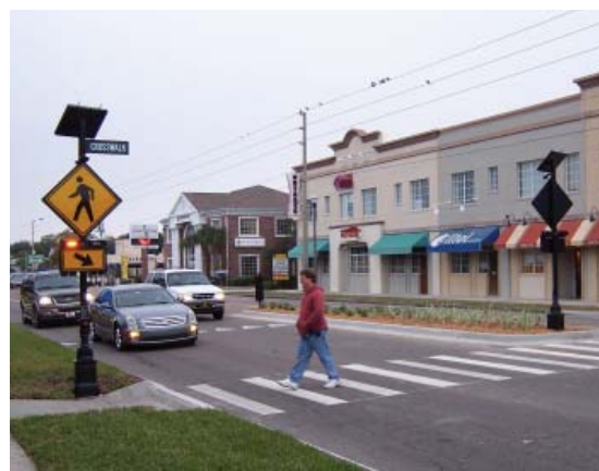
RECTANGULAR RAPID FLASHING BEACON (SOURCE: WWW.PEDBIKEIMAGES.ORG/MF )
