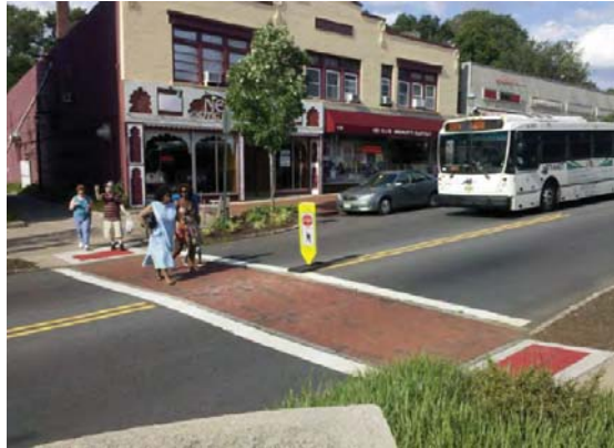
TEXTURED CROSSWALK WITH IN-STREET PEDESTRIAN CROSSING SIGN
