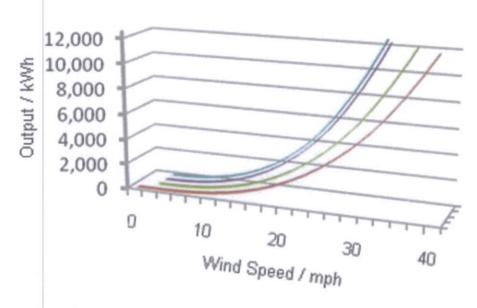
As can be seen from the graph the turbine output increases exponentially with wind speed. Location is therefore extremely important, as small increases in wind speed make large increases in output. The final position will be best suited in terms of wind direction, and to optimize roof effect.
